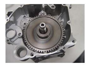
Install the starter driven gear onto the one way clutch and check for proper operation by turning the starter driven gear.
