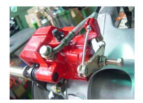
Installation is the reverse of removal. Using a C-clamp, depress the piston back into the caliper bore to provide enough room for the new pads to clear the disc.
