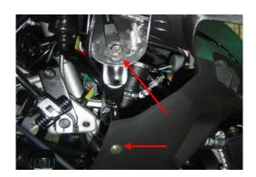
Remove fender to frame mounting bolts
