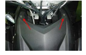
Disconnect indicator light and main switch wire. Remove L/R side cover and front to rear joint bolts.
