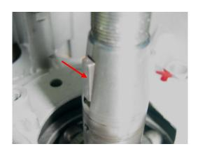
Apply molybdenum disulfide grease to the flywheel nut and crankshaft threads then install and tighten the flywheel nut while holding the flywheel.
