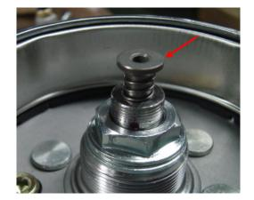
Hold the flywheel with a flywheel holder and remove the flywheel nut and washer.
