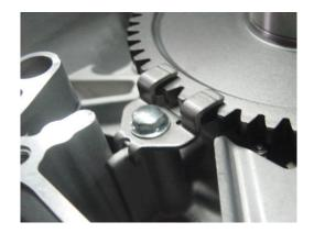
Install the flywheel onto the crankshaft, aligning the key on the crankshaft with the groove in the flywheel.
