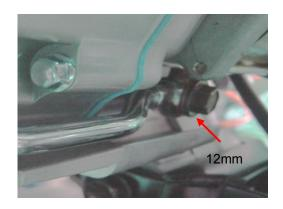
Disconnect the pulse generator and alternator wire connectors.
